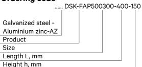
Sample: DSK-FAP500300-400-150 – made of galvanized steel sheet s bend for smoke duct sections, dimensions WxH- 500x300 mm, length 400 mm, height h 150 mm.
