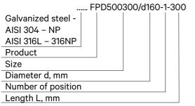
Sample: FPD500300/d160-1-300 – made of galvanized steel transition, dimensions WxH- 500x300 mm, to diameter 160 mm, centre position 1, length 300 mm.
