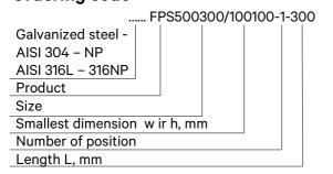
Sample: FPS500300/100100-1-300 - made of galvanized steel transition, dimensions WxH- 500x300 mm, to wxh -100x100 mm, centre position 1, length 300 mm.
