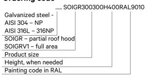
Sample: SOIGR300300H400RAL9010 – made of galvanized steel, roof hood, dimensions WxH 300x300 mm, 400 mm height, painted RAL9010.
